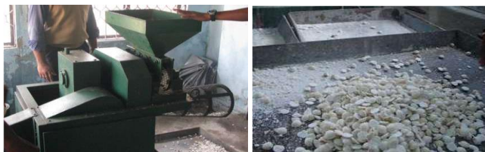
Urea briquettes/urea pellets prepared from granular urea in briquette/pellet making machine (breaking 25-30%)
